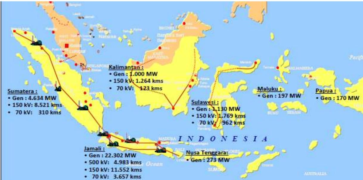
Fig.4. Indonesian electrical grid size and interconnections
